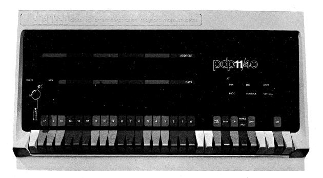
Figure 3-1a PDP-11/40 Programmer's Console
