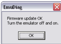
FIGURE 9 After a firmware upload, power-cycle the unit.
