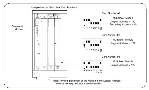
Figure 1-4. Card Numbers in a Multiple-Module Switchbox
