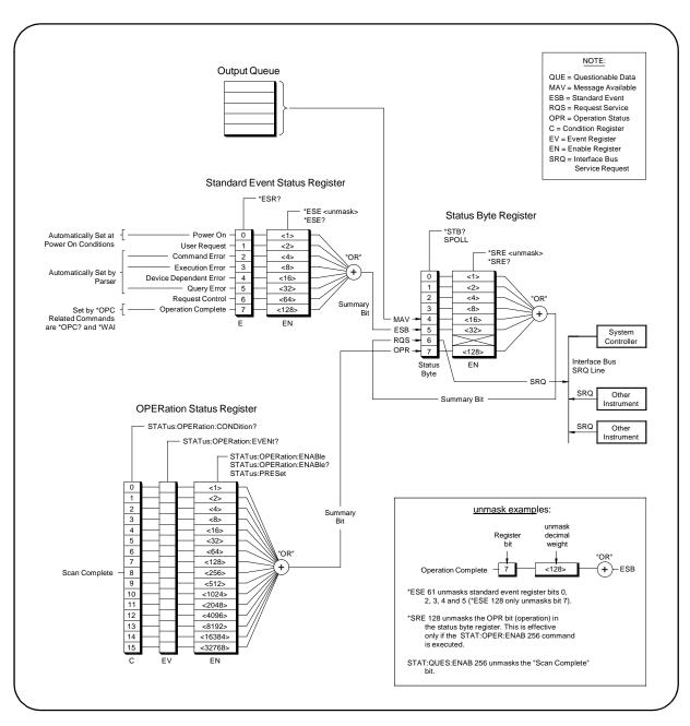
Figure 4-1. E1465A/E1466A/E1467A Status System Register Diagram
