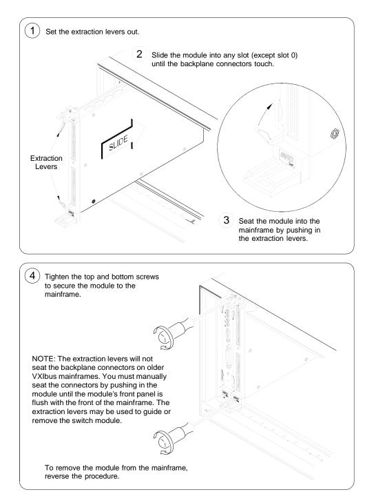
Figure 2-4. Installing the Switch Module in a VXIbus Mainframe
