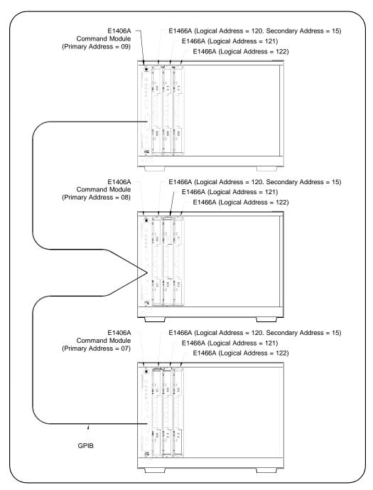
Figure 2-14. Creating Larger Matrixes with Multiple Mainframes
