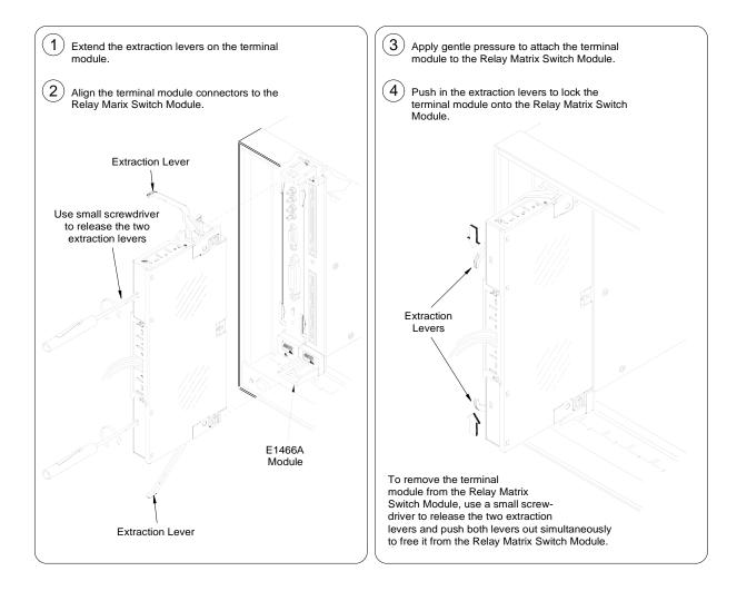
Figure 2-10. Attaching the Terminal Modules to the Switch Module
