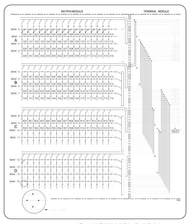
Figure 1-3. E1467A 8x32 Relay Matrix Module
