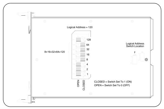
Figure 2-2. Setting the Module Logical Address
