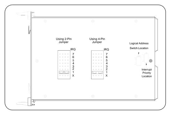
Figure 2-3. Setting the Interrupt Level
