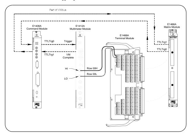
Figure 3-1. Example: Scanning Using TTL Triggers
