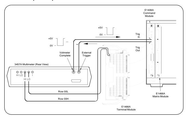
Figure 3-2. Example: Scanning Using Trig In and Trig Out Ports
