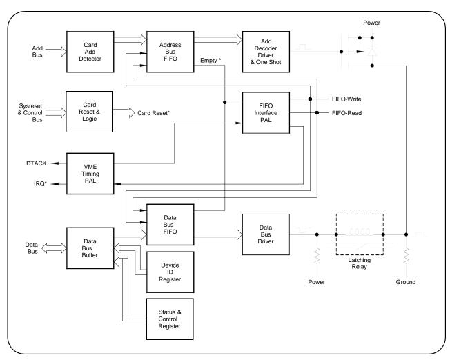
Figure 3-3. Matrix Modules Block Diagram
