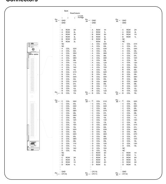
Figure 2-1. Relay Matrix Switch Module Pin-out
