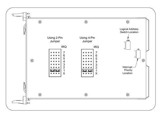
Figure 1-5. Setting the Interrupt Priority
