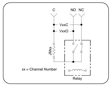
Figure 1-13. Adding Relay and Circuit Protection
