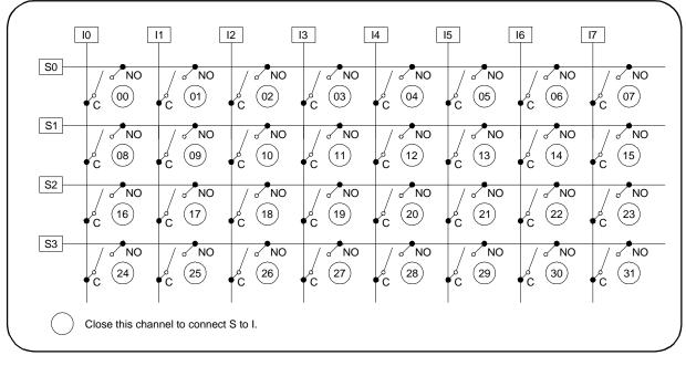
Figure 2-4. Example: Matrix Switching
