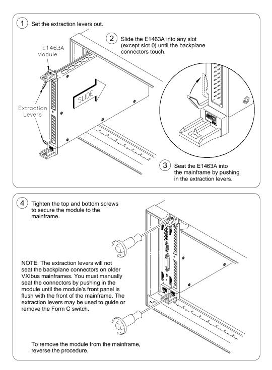
Figure 1-6. Installing the Form C Switch in a VXIbus Mainframe
