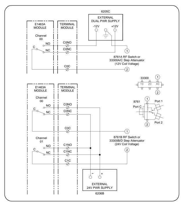
Figure 2-2. Example: Controlling RF Switches/Step Attenuators
