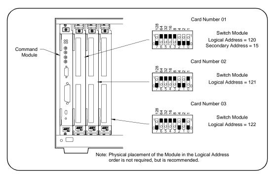
Figure 1-15. Typical Card Numbers in a Multiple-module Switchbox
