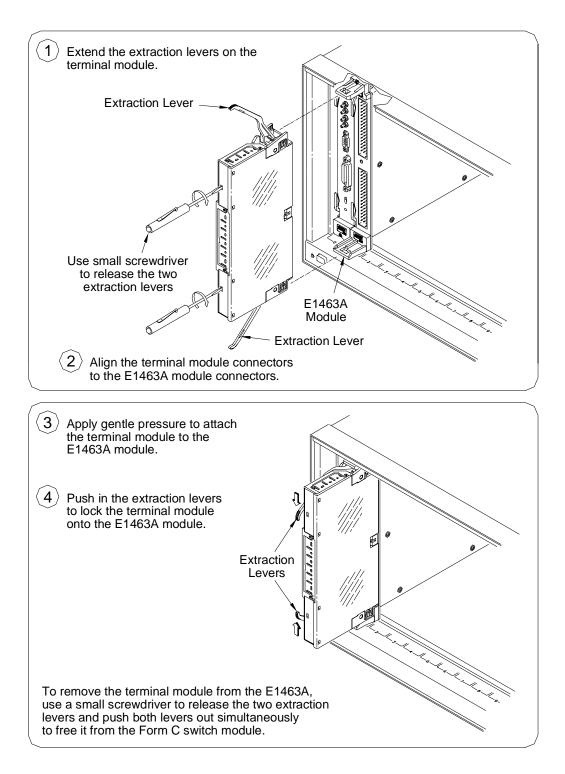
Figure 1-12. Attaching a Terminal Module to the Form C Switch
