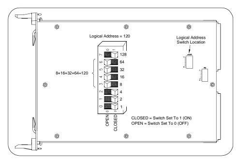
Figure 1-4. Setting the Logical Address Switch
