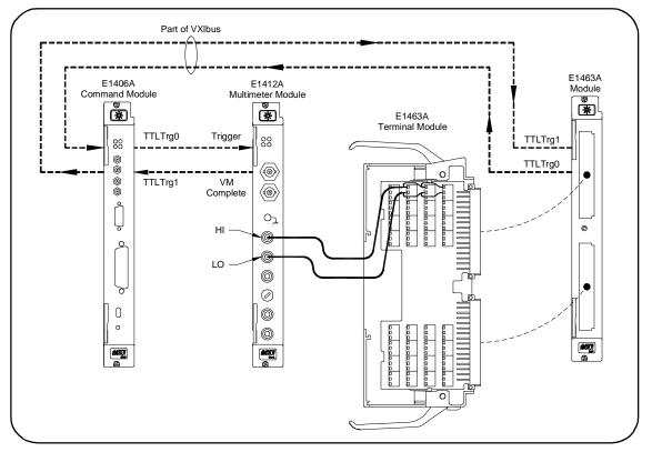
Figure 2-6. Example: Scanning Using the TTL Trigger Bus
