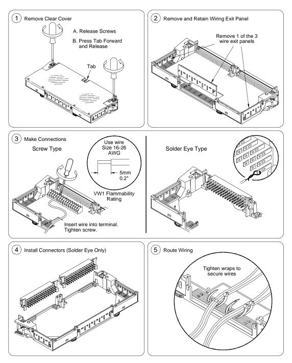
Figure 1-10. Wiring a Terminal Module (continued on next page)
