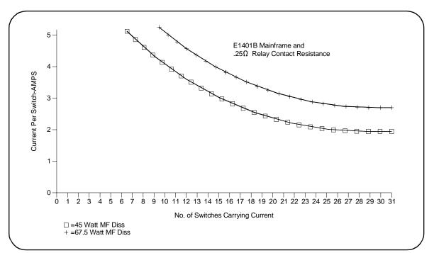
Figure 1-14. Typical Form C Switch Allowable Switch Current
