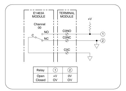
Figure 1-3. Digital Output Configuration
