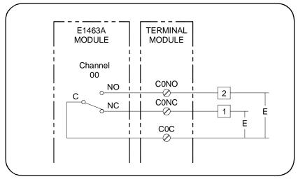
Figure 2-1. Example: Voltage Switching
