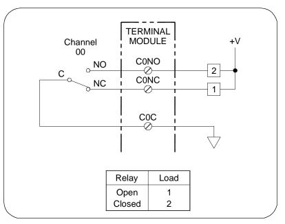
Figure 1-2. General Purpose Relay Configuration
