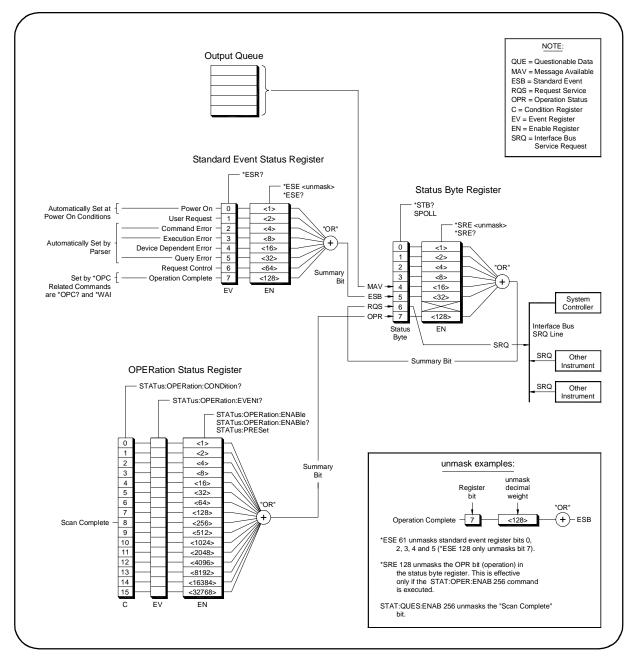
Figure 3-1. E1463A Status System Register Diagram
