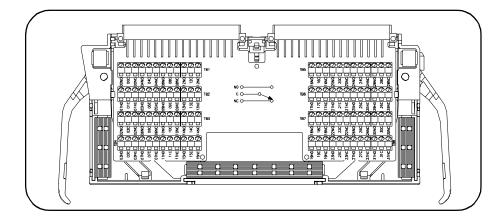
Figure 1-7. Standard Screw-type Terminal Module
