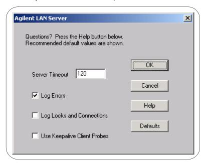
Example: Configuring LAN Server Interface The LAN Server interface system in the following figure consists of a Windows PC acting as a LAN client, a second PC acting as a LAN server, and a GPIB instrument. The IO Config utility has been used to assign the LAN card a VISA name of "TCPIPO" and SICL name of "lan". Also, the GPIB card in the LAN server PC has been assigned VISA name of "GPIBO" and SICL name of "hpib7". The LAN server PC has been assigned a name of machine2.
