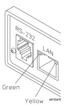
The yellow LED, on the right side of the connector, indicates LAN activity (receive or transmit).
