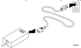
${f 3}$  Connect the 12V power cord to the back of the emulation probe.
