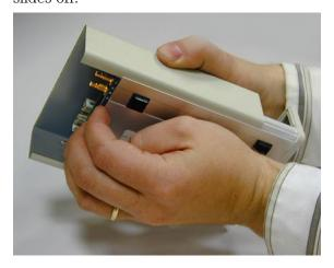
**4** Remove the 3 nylon screws from the target board adapter.
