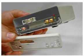
**c** Grasp the top cover with one hand. With the other hand, pull the plate on the bottom of the emulation probe, so that the top cover slides off.
