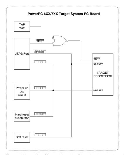
The emulation probe adds capacitance to all target system signals routed to the JTAG debug port connector. This added capacitance may increase the rise time and/or fall time of the reset signals beyond target processor specifications. Decreasing the value of the pull-up resistor on a line will decrease its rise time.
