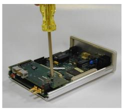
**5** Carefully lift the target board adapter from the main circuit board.
