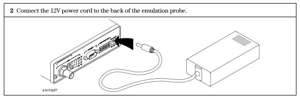
The power lamp on the target side of the emulation probe will light. The emulation probe does not have an On/Off switch.
