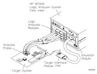
You can connect the emulation module to a debug port on the target system through the provided target interface module (TIM).
