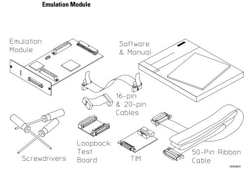
Equipment Supplied with the Agilent Technologies E3497A Emulation Module
