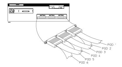
Use this table to connect cables from your target system headers to the analyzer. The table is oriented similar to the analyzer's back panel.
