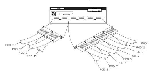
To connect to a 16600A logic analyzer
