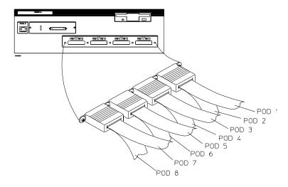
Use this table to connect cables from your target system headers to the analyzer. The table is oriented similar to the analyzer's back panel.
