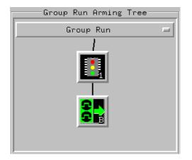
Clicking the **Group Run** button (at the very top of the Intermodule window or a logic analyzer window) will start the analyzer running. The analyzer will then wait for an arm signal. Now when the emulation module transitions into Monitor from Running (or from Reset), it will send the arm signal to the analyzer. If the emulation module is In Monitor when you select **Group Run**, you will then have to go to the emulation module or your debugger interface and manually start it running.
