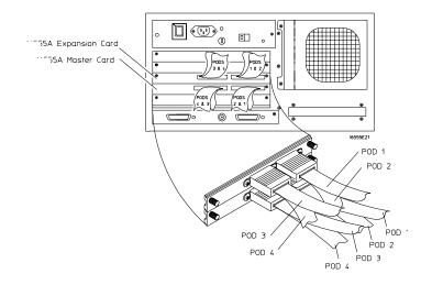
Use these tables to connect cables from your target system headers to the analyzer. The tables are oriented similar to the analyzer's back panel.
