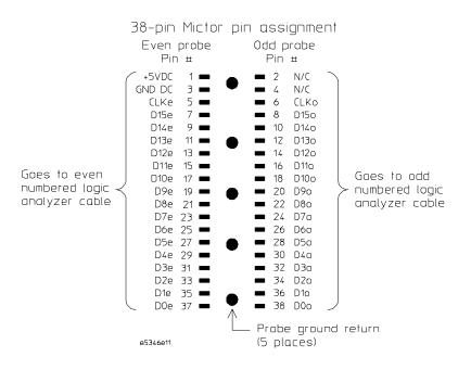
The logic analyzer signal pinouts of the high-density connector are:
