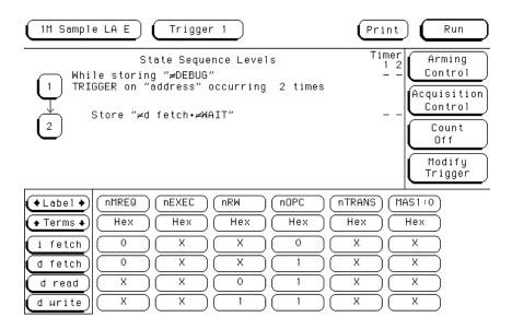
Included in the logic analyzer configuration files are several predefined trigger terms to simplify trigger setup.
