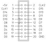
These are the pinouts for the medium-density connector header:
