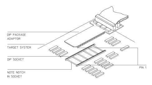
Chapter 3: Plugging the Emulator into Target Systems **To plug-in the HP 64744 emulator**
