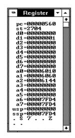
The Register window opens and displays the register contents. The display is updated periodically. To run the program and see how the contents of the registers change:
