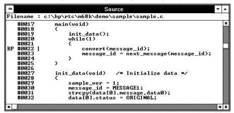
Notice that line 22 is marked with "BP," which indicates a breakpoint has been set on the line.
