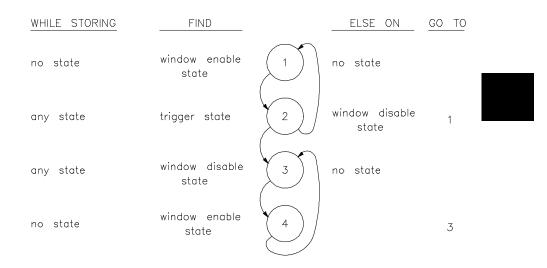
Notice that the order of the second sequence level pair is swapped. In sequence level 2, if the analyzer finds the trigger condition while searching for the window disable state, it will branch to sequence level 3 where it continues its search for the window disable state. After this, the analyzer will remain in sequence levels 3 and 4 until the trace memory is filled, completing the trace.
