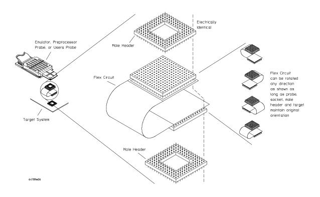
Chapter 4: Plugging the Emulator into a Target System **No-Intrusion Plug-In**
