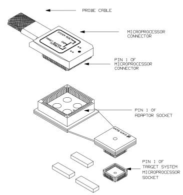
Figure 3-4. Installing into a 70136 QFP type socket
