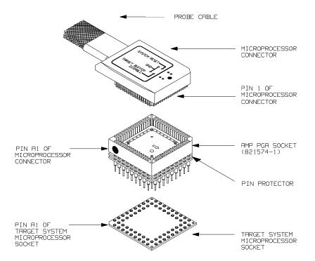
Figure 3-3. Installing into a 70136 PGA type socket
