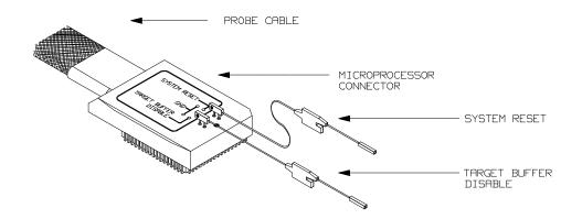
Figure 3-1. Auxiliary Output Lines (70136 Emulator)
