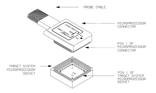
Figure 3-2. Installing into a 70136 PLCC type socket
