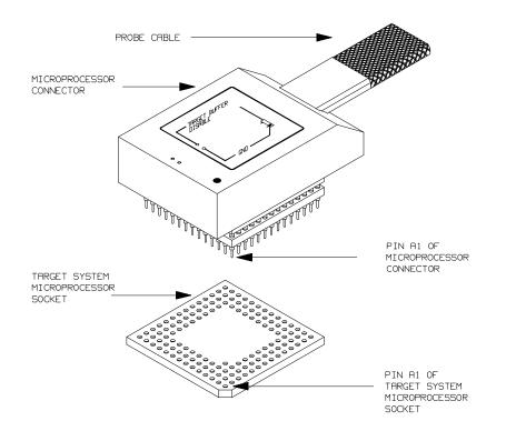
Figure 3-5 Installing into a 70236 PGA type socket
