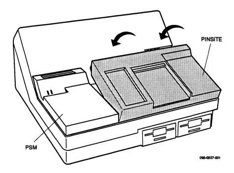
4. To remove the module, lift the rear of the module until the retaining hooks on the front of the module are disengaged from the slots on the top of the UniSite.
