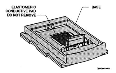
Properly maintained pads will ensure reliable performance for over 10,000 insertions for each package size 20 to 84 pins.
