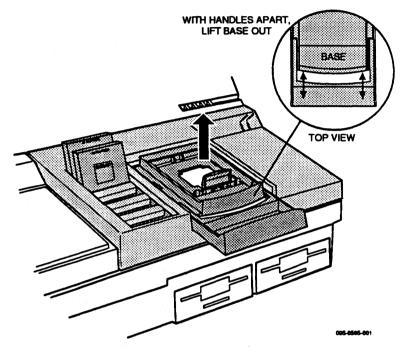
Lift the Base up and out of PinSite. Store the Base in the storage container you received with your PinSite.
