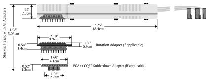
The CodeICE 060 probe tip. Dimensions are in inches.
