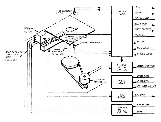
Figure 1-2 TM848 Disk Drive Functional Block Diagram
