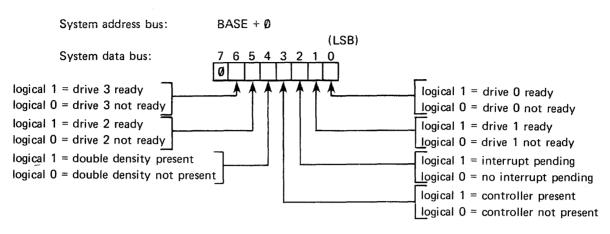
These indications allow the operating system to monitor the operation of the Controller Channel.
