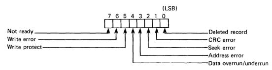
If the type code = 10, the controller has detected a change in the ready status of a drive and the contents of the result byte will indicate the current ready status of the diskette drives:
