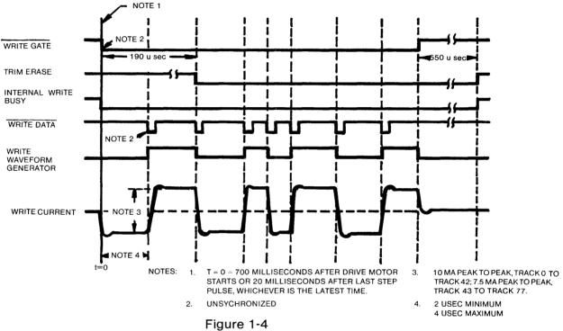
Write Operation Timing Diagram
