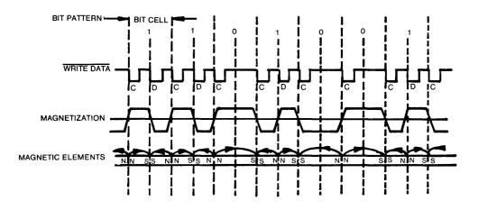
Figure 1-3 FM Recording Magnetization Profiles
