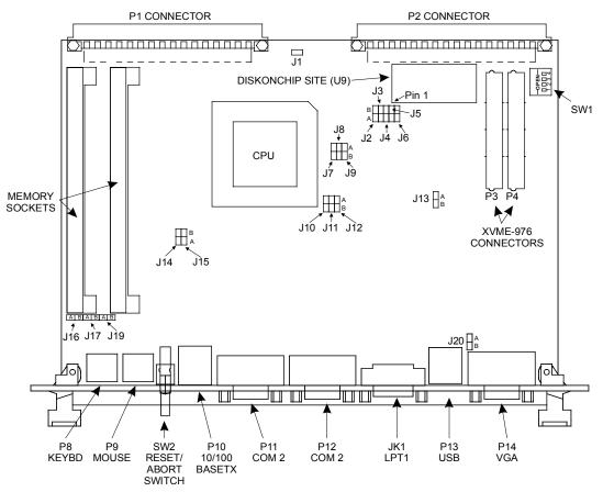
Figure 2-1 XVME-653/658 Jumper, Switch, and Connector Locations
