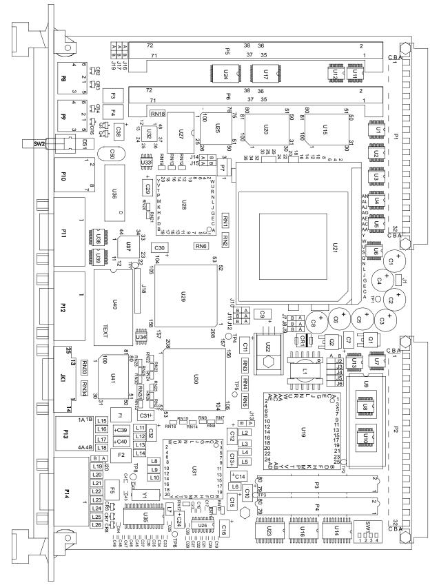
Figure B-2 Assembly Drawing for XVME-653/30x
