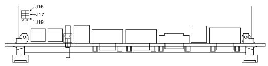
Figure 2-2 J16, J17, and J19 Jumper Locations for XVME-653/30x (no byte-swapping hardware)
