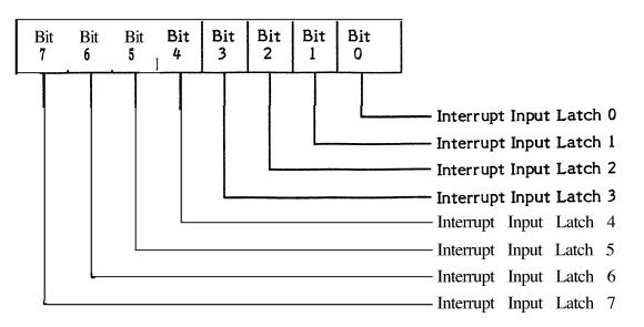
Figure 3-5. Interrupt Clear Register
