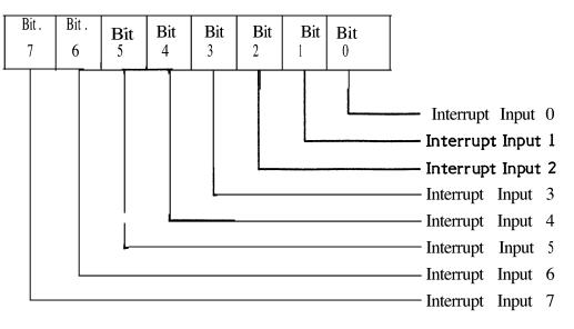
Figure 3-4. Interrupt Input Register
