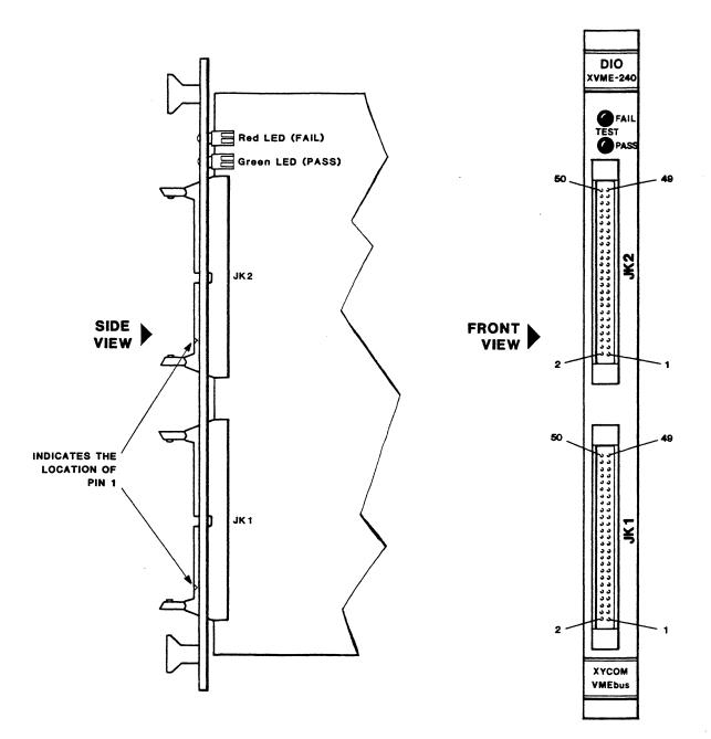
Figure 2-6. Connector Pin Numbering Scheme
