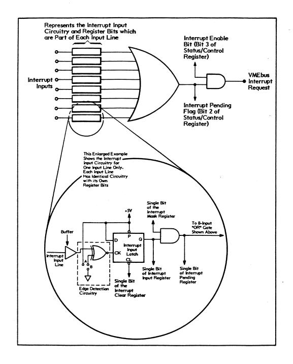
Figure 3-10. Interrupt Input Logic
