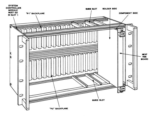
Figure 2-7. VMEbus Chassis
