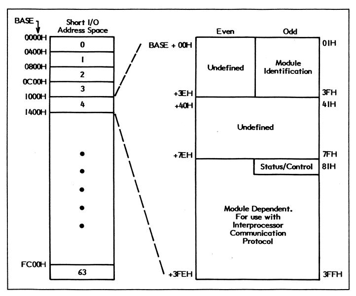
Figure A-2. XVME I/O Module Address Map
