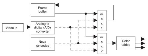
Figure 1. Block diagram of the SuperPaint memory system. Solid lines show the paths used during static display. Courtesy of Richard Shoup.
