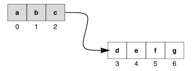
Figure 7-2 shows the same zbuf, but it is labeled with offsets relative to the second segment. This is the most efficient addressing scheme to refer to bytes d, e, f, or g in the figure.
