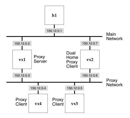
The following is an example of **vx2**'s routing table. The routing table is manipulated using **mRouteAdd()** and **mRouteDelete()**. For more information, see the reference entry for **routeLib**.
