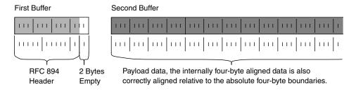
On reception, the device places the MAC header into one buffer and the payload data into the other. The driver receive function then links these together and processes them as a buffer chain in which each component buffer automatically starts on a four-byte boundary. Therefore, when the driver hands the buffer chain up to the MUX, the payload data is correctly aligned.
