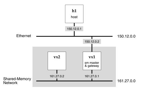
The shared memory master is **vx1**, and functions as the gateway between the Ethernet and shared-memory backplane networks. It therefore has two Internet addresses: 150.12.0.2 on the Ethernet network and 161.27.0.1 on the shared-memory backplane network.
