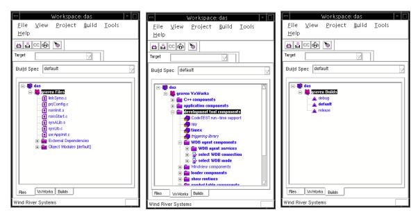
Figure 4-1 Workspace Window Views: Files, VxWorks, and Builds
