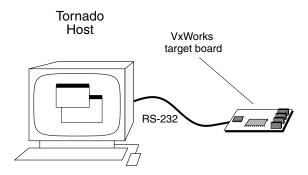
Tornado can operate over a raw serial connection between the host and target systems, and can operate on standalone systems that have no network connection to other hosts.
