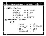
Having diagnosed the problem as a classic priority inversion, the fix is straightforward. As described in *VxWorks Programmer's Guide: Basic OS*, you can revise the application to synchronize **uLow** and **uHi** with a mutual-exclusion semaphore created with the **SEM\_INVERSION\_SAFE** option.
