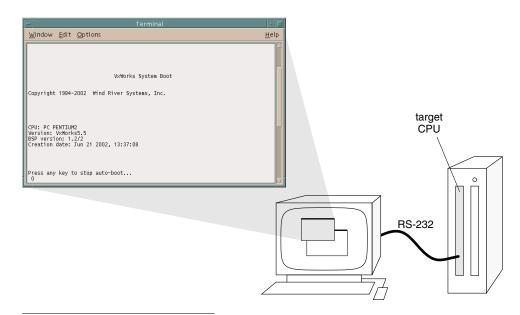
5. Unless your target CPU has nonvolatile RAM (NVRAM), you will eventually find it useful to build a new version of the boot loader that includes all parameters required for booting a VxWorks image (see 4.8 *Configuring and Building a VxWorks Boot Program*, p. 164). In the course of your developing an application, you will also build bootable applications (see 4.5 *Creating a Bootable Application*, p. 147).
