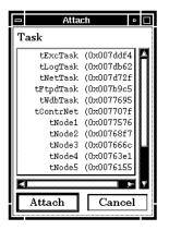
Usually, a newly-attached task stops in a system routine; thus, the debugger displays an assembly listing in its program-display panel. Use the up-stack button 1 to view a stack level where source code is visible, or use the finish button 2 to allow the system routine to return to its caller.
