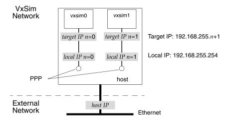
Addressing is according to processor number, such that when you run VxSim with processor number n (with the command **vxWorks -p** n), the network addresses packets as shown: .
