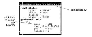
Figure 8-6 shows a binary semaphore with one blocked task in its queue. As in other browser windows, you can click on the folders to control detail. To start a
