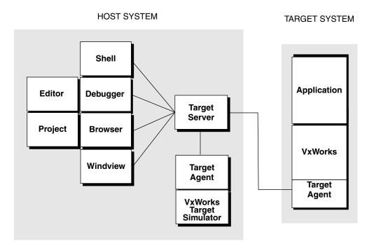
The *run-time system* (often called simply the *run-time*) is the code that is intended for the final application, as distinguished from the complete Tornado cross-development environment. The run-time includes the real-time kernel, and typically also includes some selection of VxWorks library code as well as application-specific code. It does not usually include the target agent, although in some cases the target agent can be included to provide field debugging.
