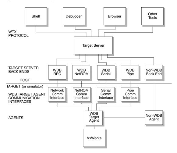
Figure 2-1 Tornado Host-Target Communication
