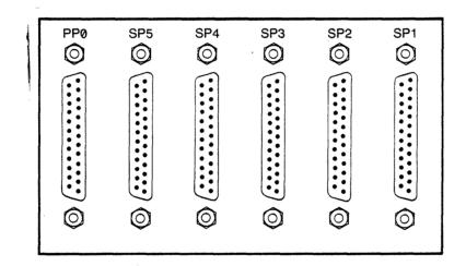
Use ports 1 through 5 to connect terminals to the CPU for a 150-6 configuration. Ports 1 and 2 should be used for the 150-3. Complete detail on pin connection, etc., is provided in the System 150 (mapped) Hardware Reference Manual.
