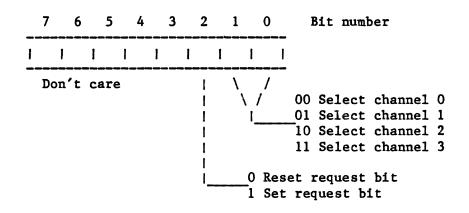
Software requests are serviced only if the channel is in Block mode.
