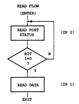
Figure 6.2B Read Flow Diagram
