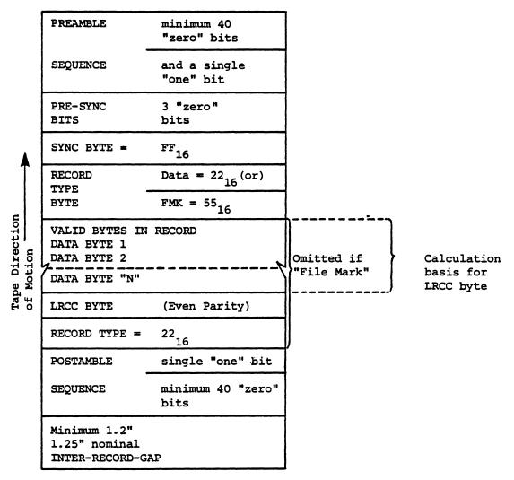
NOTE: All bytes consist of 8 data bits (LSB first) 1 vertical parity bit (even)
