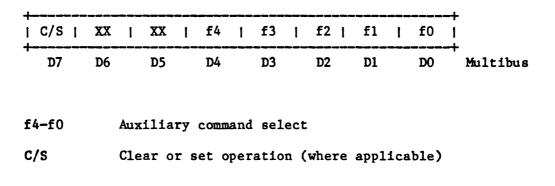
Auxiliary commands entail many special features. To carry out a function, the multibus writes data at the location corresponding to the auxiliary command register. To select the required command, load the appropriate byte as shown in table 7-C.
