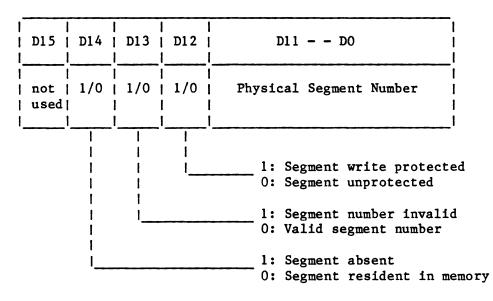
Figure 2.3 Memory Mapping Register Format
