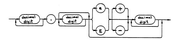
The decimal point can appear anywhere to the right of the first digit. However, a real number cannot start with a decimal point. A real number can be specified with or without an exponent.
