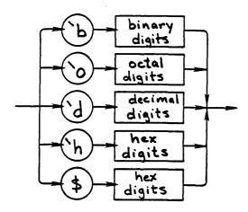
For compatibility with previous assemblers, the dollar sign (\$) can be used to specified the hexadecimal radix. The legal characters for each radix are listed below.
