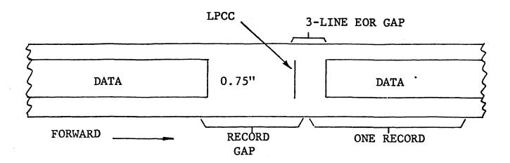
After writing the last line, the Controller writes an LPCC and an EOR gap. Minimum record gap is 0.75 inch. As shown above, the controller assembles pairs of bytes into words. Zeros appear in the unused bits.
