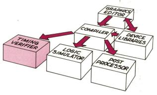
interface requirements. Timing Verification uses data that includes: estimated or actual wire delays, designer specified interface requirements and device parameters specified in component libraries. The parameters in these libraries include: propagation delays; set-up and hold times; pulse width constraints; and edge-to-edge constraints
