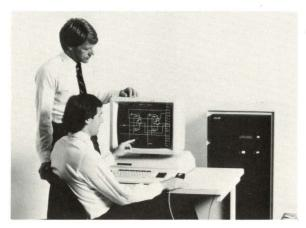
Interactive Engineering with SCALD makes it possible to design systems that are error-free. Designs are debugged before any hardware is built.
