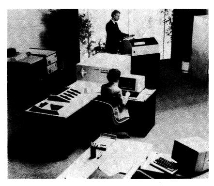
The System 80 equipment is designed for use either in a computer room or in a controlled office environment. In addition to the standard console workstation in the center of the photo, up to 39 CRT workstations such as the one at lower right can be cable-connected to the system at distances of up to 5000 feet.
