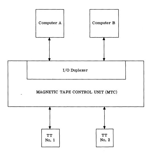
Figure D9-1. Block Diagram of Magnetic Tape System
