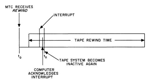
Figure D9-7. Execution of Rewind Function
