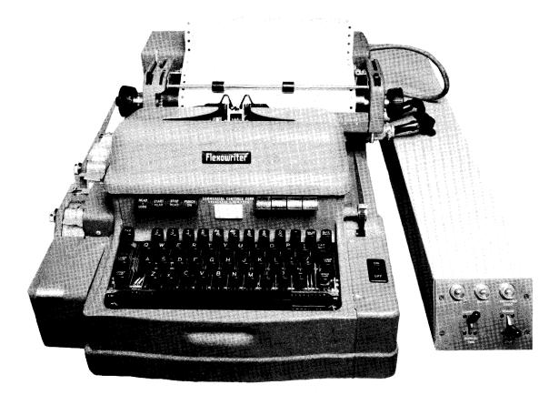
Figure D5-1. Monitoring Typewriter (Flexowriter, Model FL)
