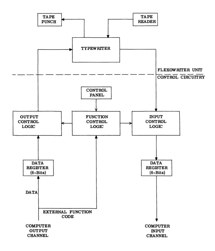
Figure D5-3. Block Diagram of Monitoring Typewriter
