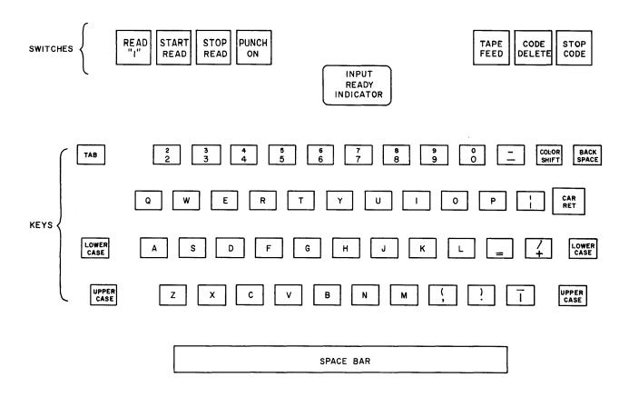
Figure D4-1. Keyboard Layout of Monitoring Typewriter
