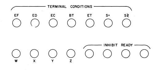
A TERMINAL CONDITION CAN BE PATCHED EITHER TO ONE OF THE W,X,Y, OR Z JACKS, OR TO AN INHIBIT READY JACK
