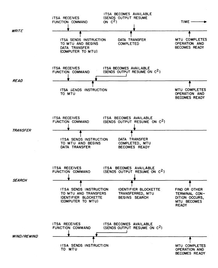
Figure D1-6. Tape System Operations
