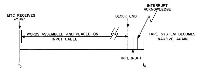
Figure D9-5. Execution of *Read* Function
