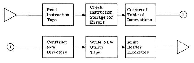
Figure E1-5. Block Diagram of Utility System Update Program
