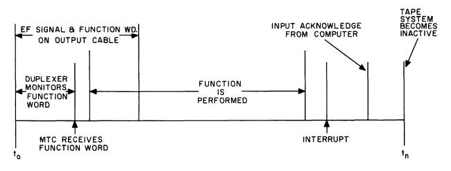
Figure D9-2. Timing of Function Word Performance
