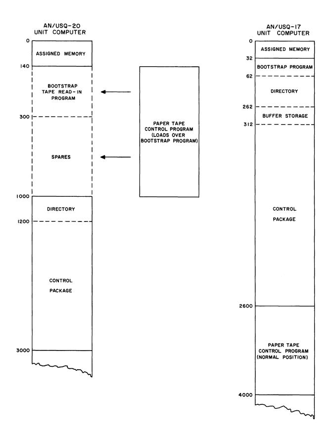
Figure E1-12. Locations of Control Package and Paper Tape Control Program in Core Memory
