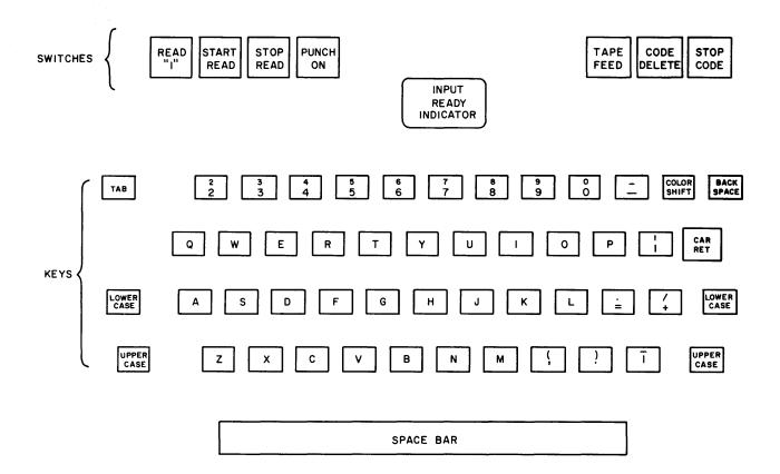
Figure D5-2. Monitoring Typewriter - Keyboard Layout
