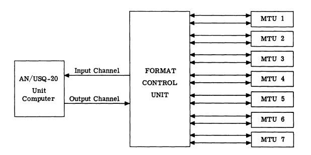
Figure D10-1. Interconnections of Tape System Equipment
