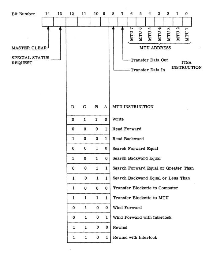
Figure D1-2. Function Command Word - Unit Computer to ITSA
