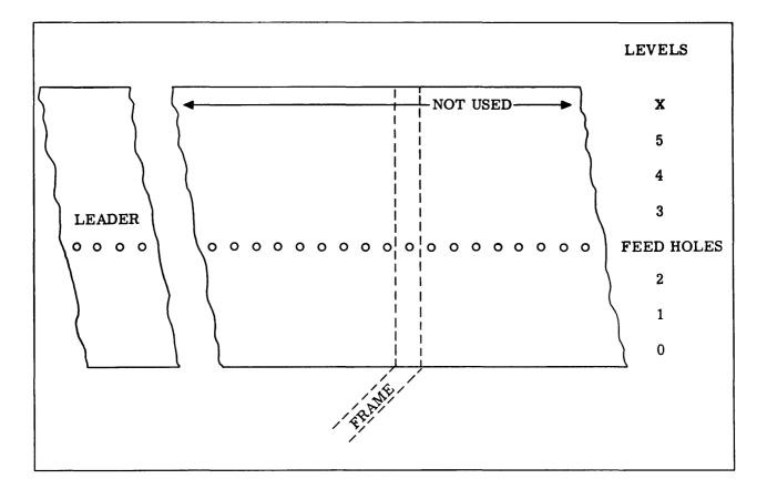
Figure D6-1. Portion of Punched Tape
