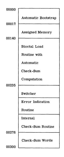
Figure E3-1. Memory Locations Used by Automatic Bootstrap and Bootstrap Tape Programs
