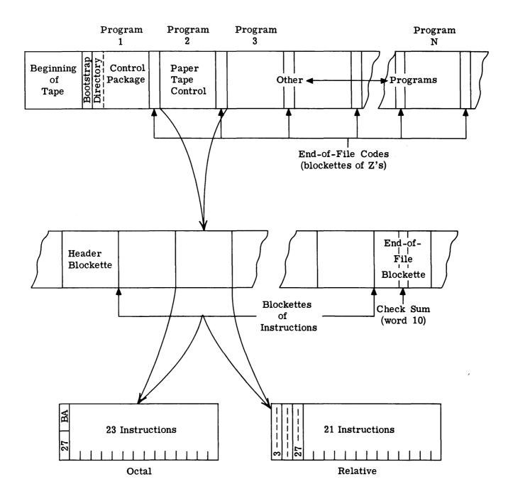
Figure E1-7. Arrangement and Format of Utility Tape
