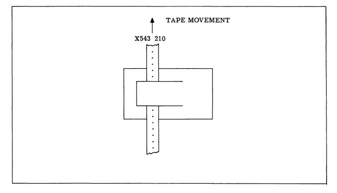
Figure D6-2. Orientation of Tape
