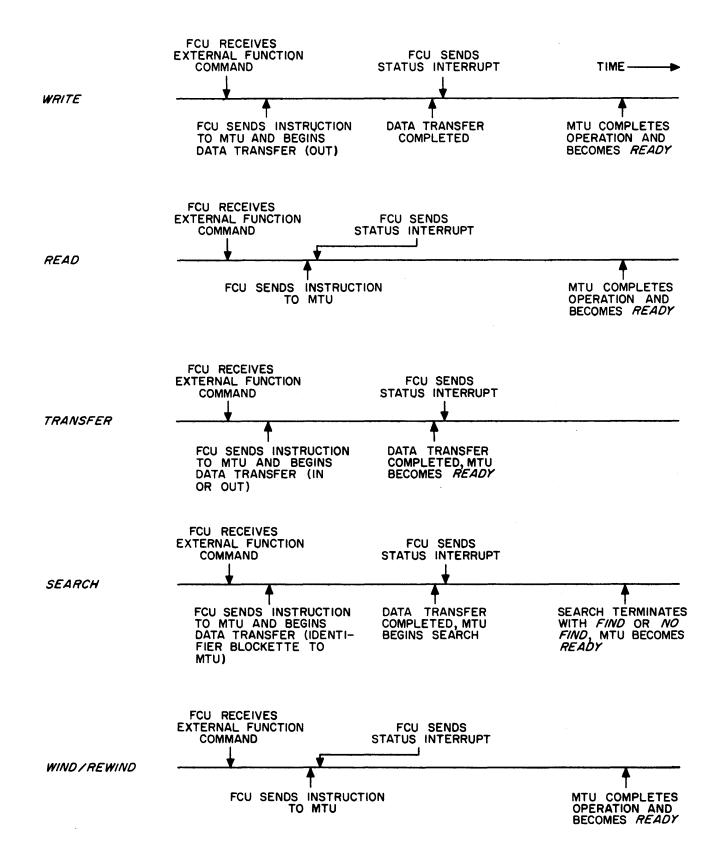
Figure D10-7. Tape System Operations
