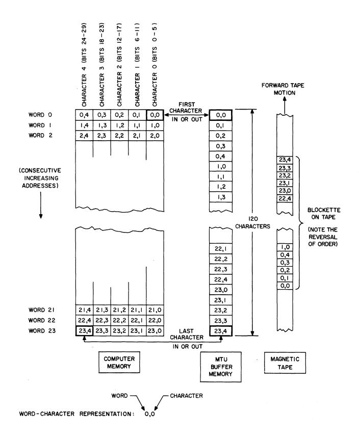
Figure D1-5. Corresponding Character Positions in Computer and MTU
