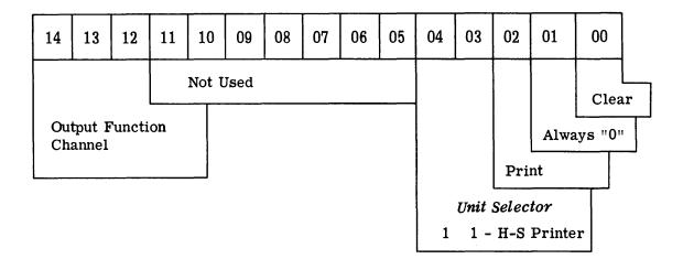
Figure D3-1. C<sup>3</sup> External Function Word
