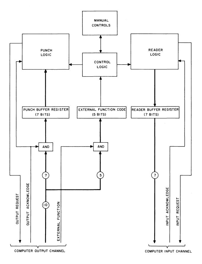
Figure D7-1. Block Diagram - Punched Tape Unit
