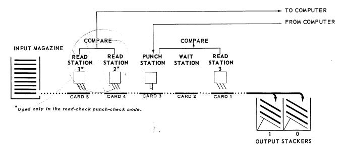
Figure 2-1. Punch-Verifier Transport System
