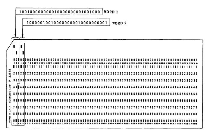
Figure 3-2. Relationship of Computer Words to Card Punches (by Column)
