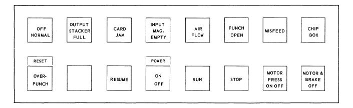
Figure 4-2. Punch Verifier Control Panel
