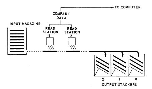
Figure 2-2. High-Speed Reader Transport System
