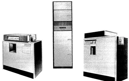
Figure 1–1. UNIVAC 490 Card Subsystem – High-Speed Reader, Channel Synchronizer-Control Unit and Punch Verifier
