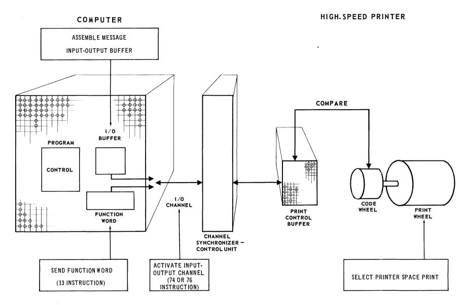
Figure 4-2. UNIVAC 490 Computer and the High-Speed Printer
