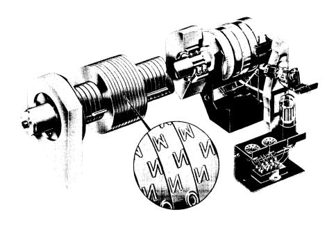
Figure 2-2. Printer Typewheels
