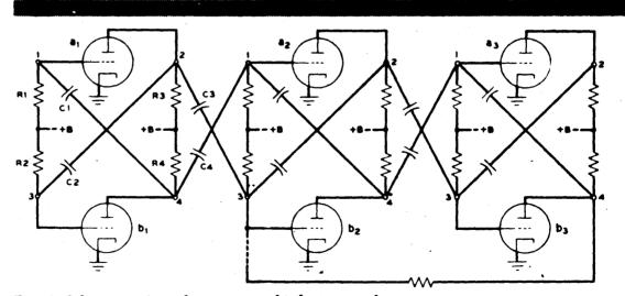
Fig. 3-Schematic of a three-stage multivibrator step-down
