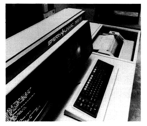
The most recent addition to the 1100 Series of large-scale sytems is the 1100/90 System. With double the main memory capacity of the 1100/60 and 1100/80, the 1100/90 provides a new virtual machine capability, and features a number of extensions to the 1100 Series architecture.
