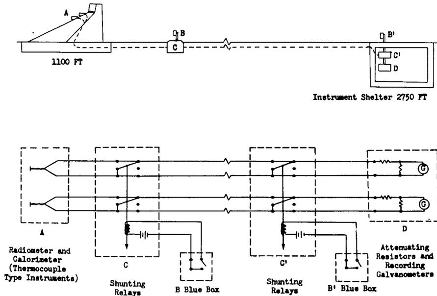
Figure 2.13 Instrumentation Schematic
