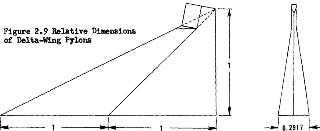
Figure 2.9 Relative Dimensions of Delta-Wing Pylons
