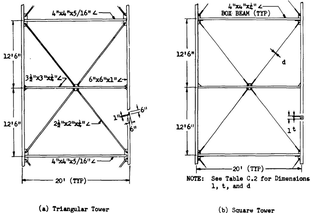
Figure C.1 Typical Tower Construction
