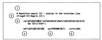
Figure 5-2. Hazeltine Esprit III Terminal Section
