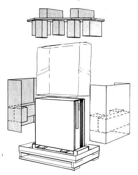
7. Move the main unit off of the box bottom and shipping pallet and place in the installation area.
