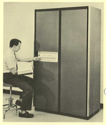
FAST Completes typical programs at a rate of a thousand operations per second, sufficient for over 90 percent of all control installations. Special design features directed toward speed of operation are automatic scanning, literal addressing, and input and output buffering. The TRW-330 is the fastest drum-memory control computer available.
