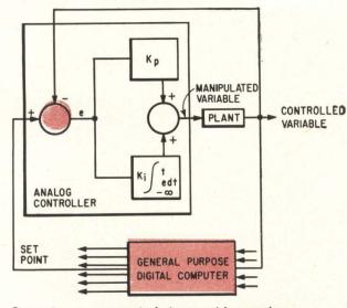
**Computer process control** at present is complex. Diagrammed is one control loop of a general purpose digital computer controlled process
