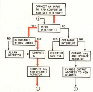
**DDC computer operation** is shown in this flow chart. Improved process control results from wider adjustment range and non-interacting parameters of signals
