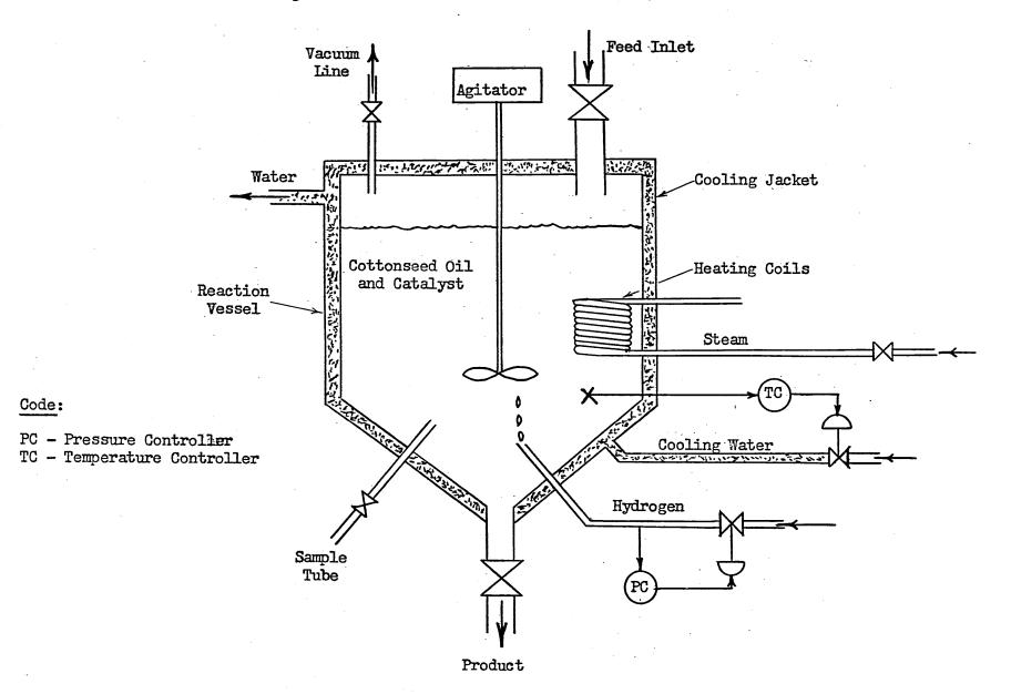
Fig. 7 CONVENTIONAL CONTROL OF HYDROGENATION PROCESS
