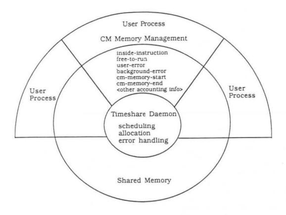
Figure 5: Timesharing control mechanism.
