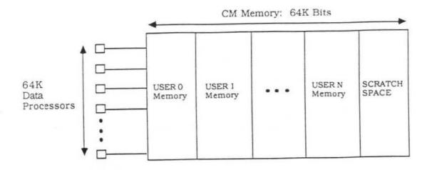
Figure 4: CM memory configuration under timesharing.
