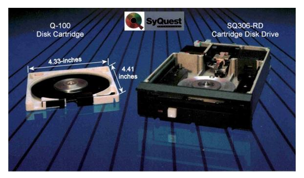
The Q-100 cartridge contained a 3.9-inch aluminum disk with a plated recording layer overcoated with sputtered carbon.
