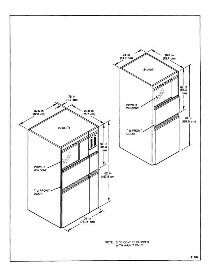
Figure 2-1. Tape Subsystem Dimensions
