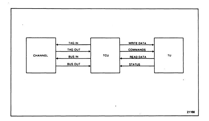
Figure 1-3. System Block Diagram
