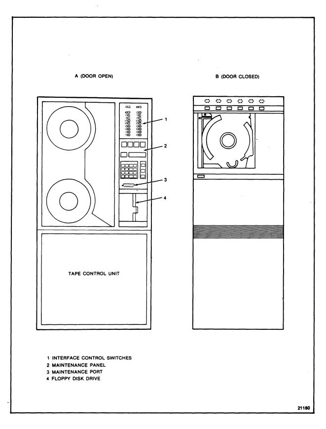
Figure 1-2. 4600 Tape Subsystem A- and B-Units
