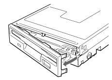
2 To remove the eject button, pull out the eject button. To insert the eject button, align the eject button with the pin and push it until it is fully inserted.
