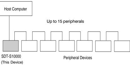
Figure 1-1. Example of System Components
