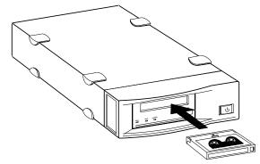
Figure 3-1. Inserting a data cartridge
