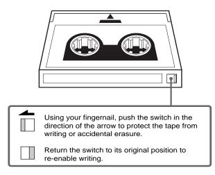
Figure 4-1. Write-protect switch
