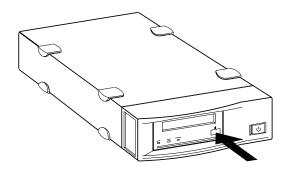
Figure 3-2. Press the EJECT button
