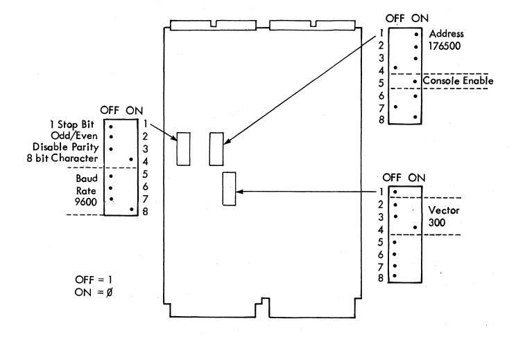
FIGURE 2-1: COMPONENT LOCATIONS SHOWING FACTORY CONFIGURATIONS
