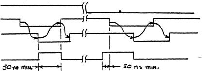
When the data transfer is to the controller, the controller will wait 50ns or more after
