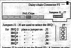
Jumper J7 is used to set the Board ID. A jumper on pins 2 & 3 indicates Board ID 0, and a jumper on pins 1 & 2 indicates Board ID 1.
