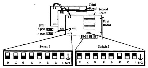
Switch 1 sets the I/O addresses for the card. The example above shows the setting for I/O address 140h. Each adapter in the system needs to have its own unique I/O address setting (see below).
