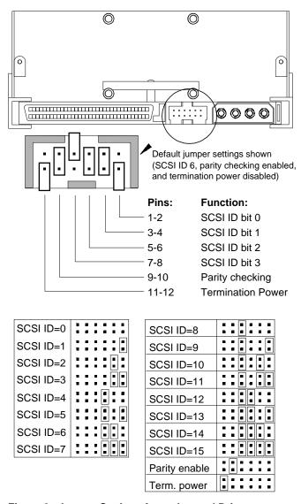
Figure 6. Jumper Settings for an Internal Drive
