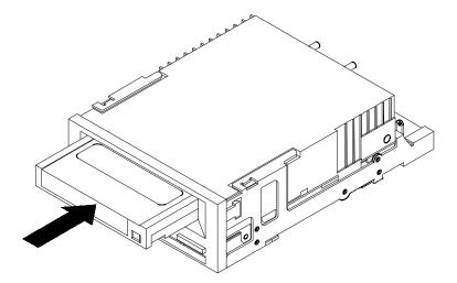
Figure 16. Loading a Tape Cartridge
