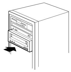
Figure 8. Mounting an Internal Drive
