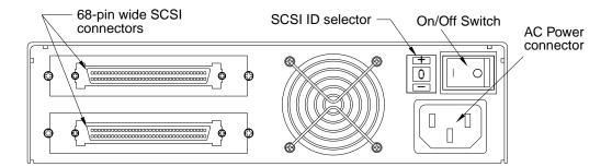
Figure 14. Rear Panel of External Drives
