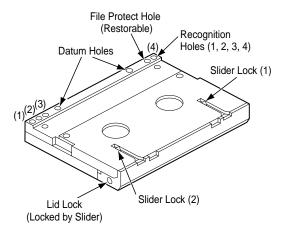
Figure 22. DDS Drive Cartridge Design Features
