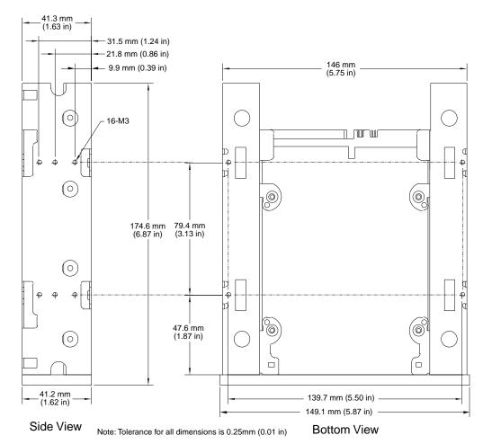
Figure 10. Mounting Holes for an Internal Drive in a 5.25-inch Configuration (with mounting brackets)
