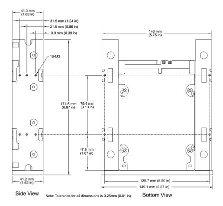
Figure 5. Internal DDS Drive with Rails—Dimensions
