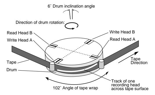
Figure 20. Four-Head Cylinder Design
