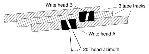
Figure 21. Alternating Azimuth Angles on Tape Tracks
