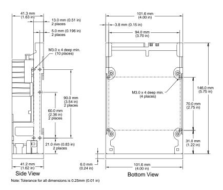
Figure 4. Internal Drive—Dimensions
