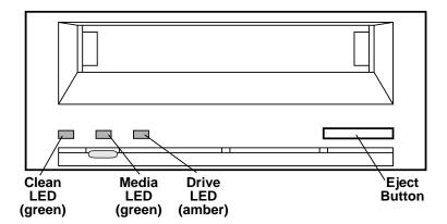
Figure 17. Location of the Eject Button and LEDs on internal Drives (external drive is similar)
