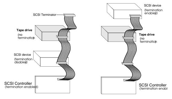
Figure 12. Two SCSI Termination Examples for Internal Drives
