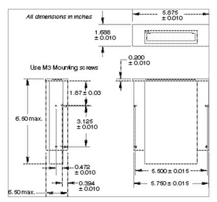
Figure 5 STT2401A (5.25-inch mount) general dimensions
