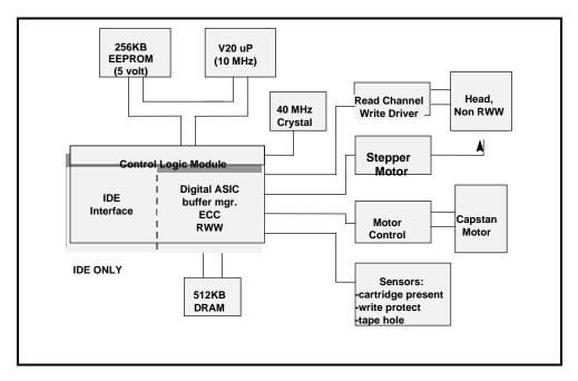
Figure 18 Simplified block diagram for STT2401A and STT3401A
