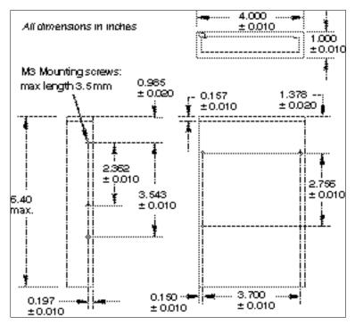
Figure 4 STT3401A (3.5-inch mount) general dimensions
