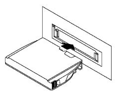
Figure 11 Loading a Travan cartridge
