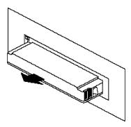
Figure 12 Unloading a Tape cartridge
