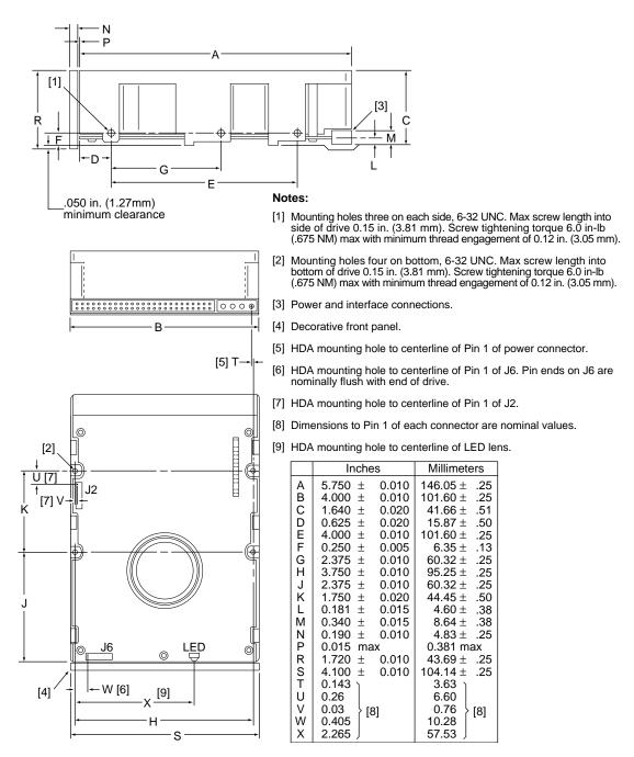
Figure 6. Mounting configuration dimensions for "N" models
