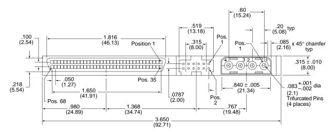
Figure 18. Non-shielded 68-pin SCSI device connector
