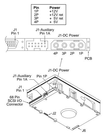
Figure 14. Physical interface for "W" and "WD" model drives (68-pin J1 SCSI I/O connector)
