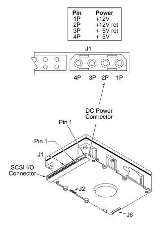
Figure 13. Physical interface for "N" model drives
