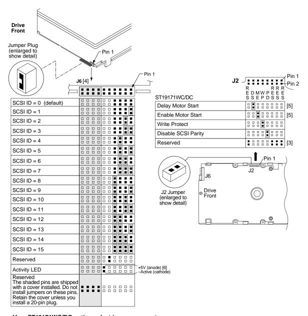
Figure 11. ST19171WC/DC option select jumper connectors
