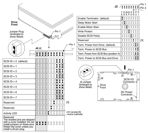
Figure 9. ST19171N option select jumper connectors
