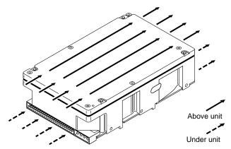
Note. Air flows in the direction shown (back to front) or in reverse direction (front to back)
