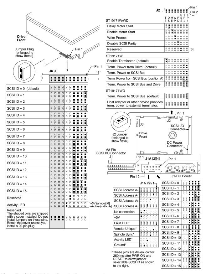
Figure 10. ST19171W/WD option select jumper connectors
