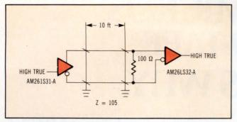
Fig 4 The data line driver/receiver combination used in the ST412 HP constitutes an EIA RS-422 driver/receiver pair, which employs flat ribbon cable or twisted-pair wiring. A proposed "Dash A" version specifies additional high performance parameters.
