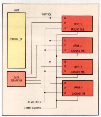
Fig 7 A typical connection for a four-drive Winchester subsystem shows the daisy chained control lines and radial data lines. Note that the data separator is part of the controller.
