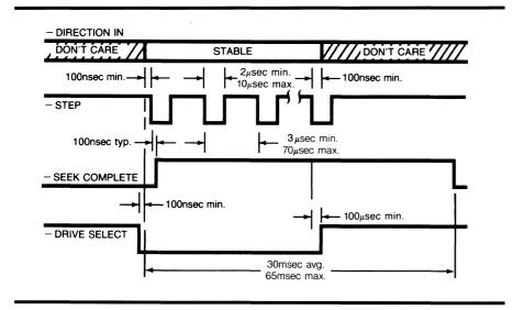
FIGURE 12: Buffered-Seek **Timing**
