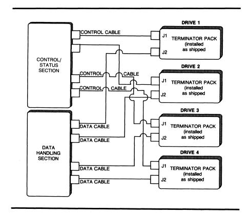
FIGURE 9: Radial Configuration
