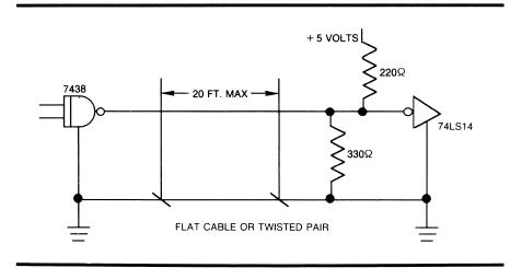
FIGURE 10: Control Signals Driver/Receiver Combination
