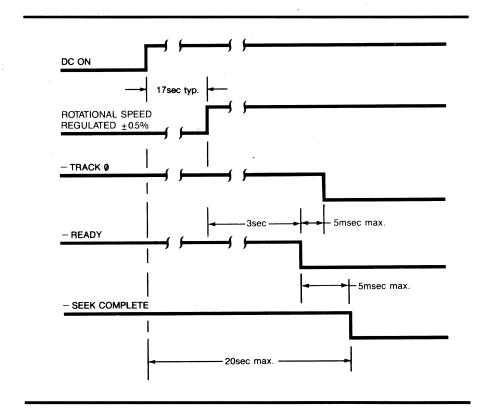
FIGURE 16: Typical Power-On Sequence
